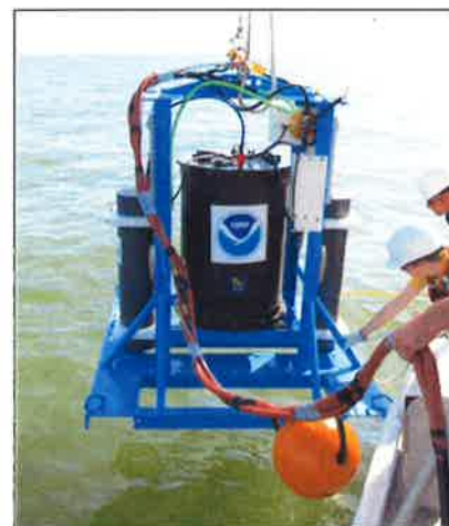
A test deployment of the ESPniagara in June 2016. Credit: NOAA.
